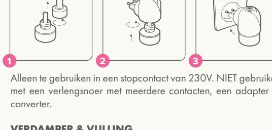
To be used with 230V plug socket only. DO NOT use with multi-socket extension cords, extension leads, an adaptor or converter.
